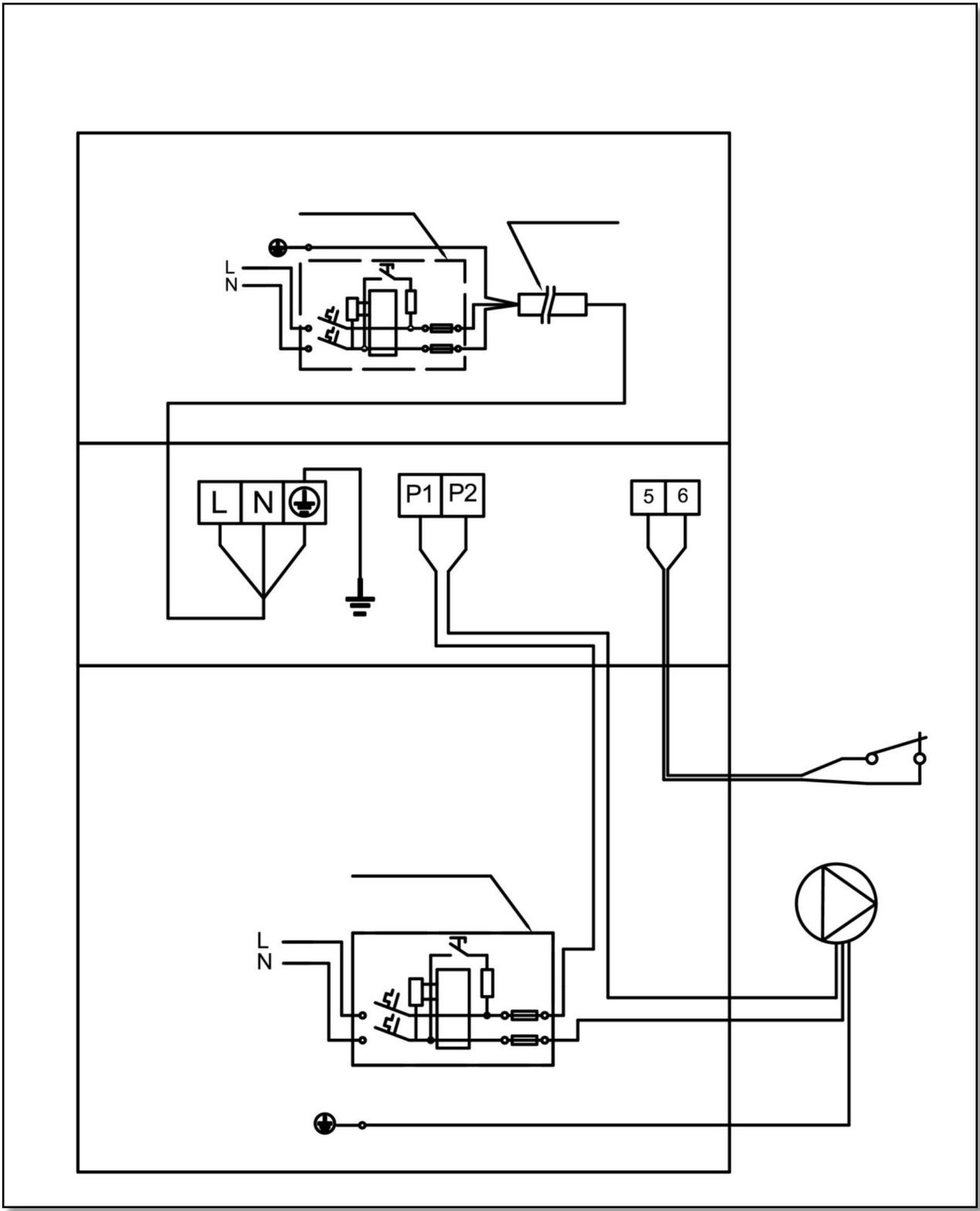
Water pump: 230V voltage, >500W capacity
